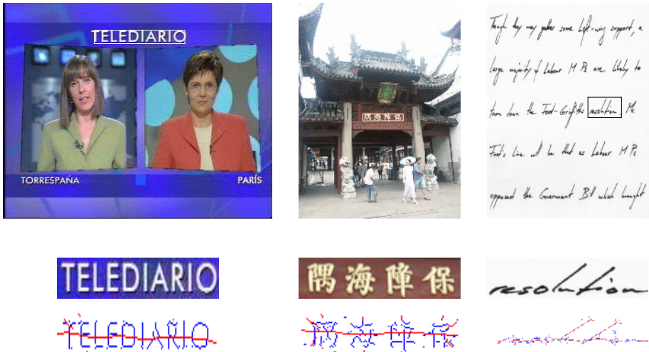
Fig. 2. First line: Images with rectangle showing the text region. Second line: Zoom on text regions. Third line: ridges detected at two scales (red in high level, blue in small level) in the text region that represent local structures of text lines whatever the type of text (handwritten text or machine text, scene text or artificial text, latin alphabet or ideograms).
