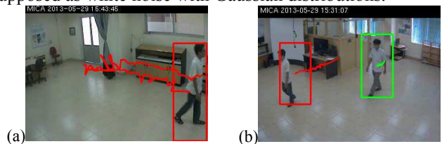
Fig. 4. (a) Tracking results: (a) Bounding box represents the current location of the human, the red line is his trajectory; (b) Each person and his trajectory are represented by a color in multiple human tracking.
