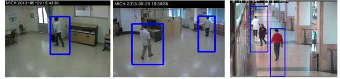
Fig. 2. Detection results obtained from differencing current frame with background frame.
