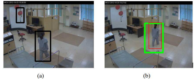
Fig. 3. (a) Detection results (black rectangles) by applying HOG-SVM on whole image. (b) Detection results (red rectangle) by applying HOG-SVM on the extended region (green rectangle). The false alarm in (a) (smaller rectangle) is now removed in (b), the localization of human is more precise.
