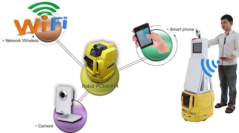
Fig. 1. The functional components of the system navigational aids visually impaired people using mobile robot
