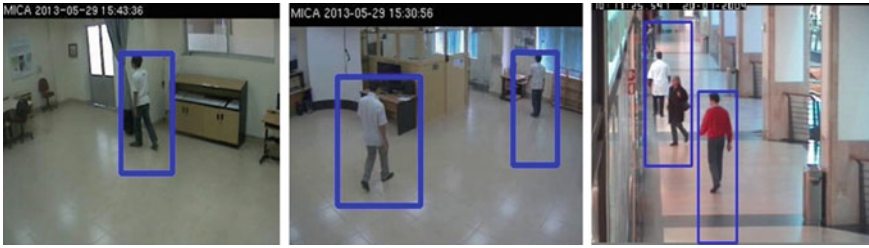
Fig. 3 Detection results obtained from differencing current frame with background frame
