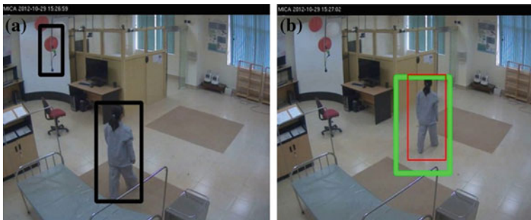
Fig. 4 a Detection results ( black rectangles ) by applying HOG-SVM on whole image. b Detection results ( red rectangle ) by applying HOG-SVM on the extended region ( green rectangle ). The false alarm in (a) ( smaller rectangle ) is now removed in (b) , the localization of human is more precise
